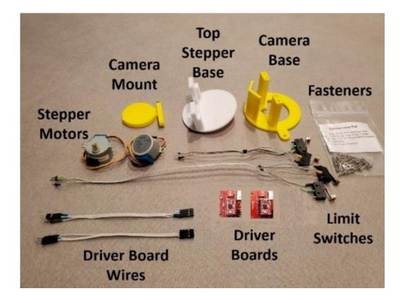
(3) Fasteners used in the assembly of the camera mount are machine screws and nuts and self-tapping sheet metal screws.
