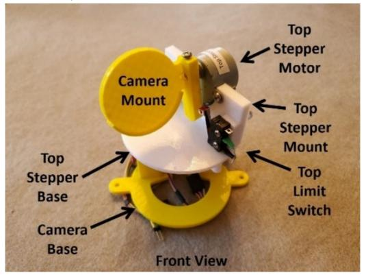
(2) Verify that your Camera Mount package has all required parts. The parts include the camera base, top stepper base, camera mount, two stepper motors – both are the same, two pairs of limit switches (top switches have long wires and bottom switches have short wires, two driver boards, one fastener package (screws and nuts), and a pair of driver board wires. The photos show the individual parts of the camera mount unit to be assembled.
